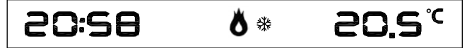
Pic.14 N.B. To know the temperature set at a specific hour, press one of the arrow keys ; on the display the actual hour and temperature (ex. H15 20°C) appear.
