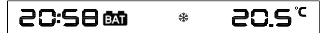
Pic.16 START UP When wired, Simply makes a control cycle lighting up all the display segments and switching the load for few seconds.
